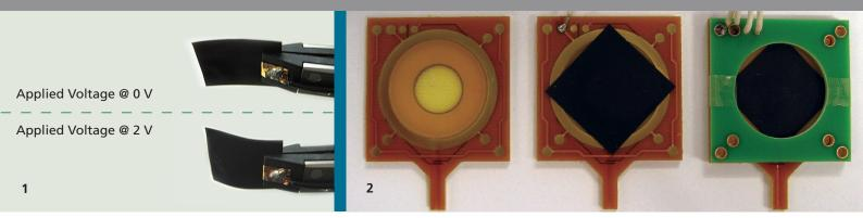
Actuation of the three-layered CNT actuator (©AIST Kansai)
