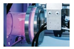
1 By means of a plasma reactor ceramic and metal nanoparticles can be specifically produced and modified.
